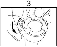
Place the fixing ring on top of the Oring on overflow tube. Lock the fixing ring.
