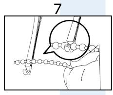
Connect bead chain to notch on the flush motor.
