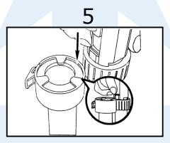
Slide the flush motor into the fixing ring
