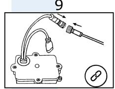
Connect the flush motor to the Host, ensure you screw collar tight once plugged in. You can now carefully place the lid back on your cistern.
