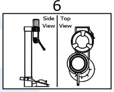
Flush motor should be as close to the top of the flusher valve as possible, allowing the bead chain to go directly to the water stop valve.
