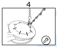
Secure the hook end of the bead chain to the water stop valve inside the toilet tank.
