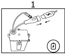
Please ensure batteries in Host are fully charged after receiving the goods. Charge time is around 4-5 hours, the light will be on solid blue when fully charged.
