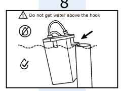
Hang or Zip Tie Host into the drain hole of the toilet cistern, do not to get wet above the hook. Please also ensure rubber stopper is installed on Host, to prevent water getting inside.
